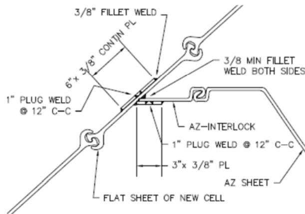
**Figure 6. Detail showing interconnecting knuckles of flat sheets, and the reinforcement used to strengthen the junction pile “Y” connector**
