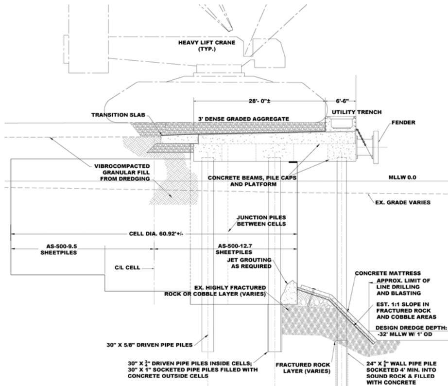
**Figure 3. Final design section of deeper draft bulkhead (dredging to -32, stepped circular cells, overhanging pile supported platform and toe scour protection).**
