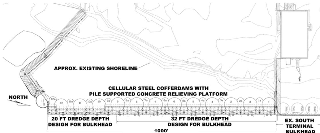
**Figure 2: Cellular Steel Cofferdams and Pile Supported Relieving Platform**
