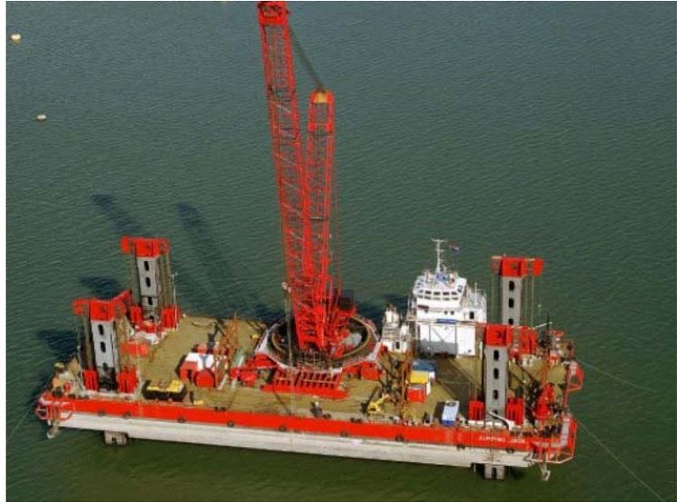
Figure 16: Jumping Jack Barge for Offshore Wind Farm Installation<sup>24</sup>
