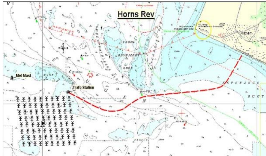
Figure 15: Horns Rev Project Layout<sup>22</sup>
