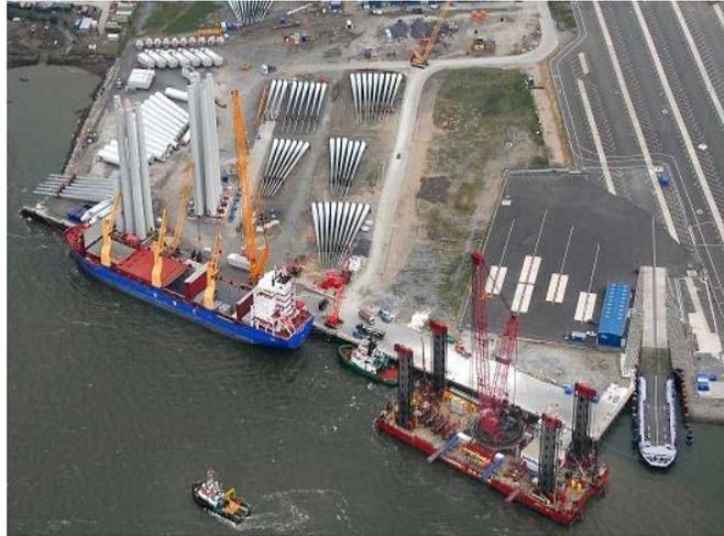
**Figure 18: Port of Mostyn Construction Base for Burbo Bank Offshore Wind Farm (UK)<sup>28</sup>**
