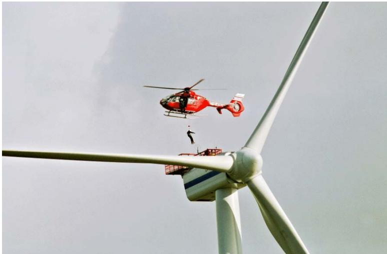
**Figure 19: Helicopter Access to Vestas Turbine<sup>29</sup>**
