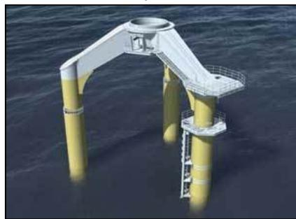
strength and wider footprint created by the three piles is expected to allow for turbine installation in water up to 50 meters in depth. The tripile design is easily adaptable to a variety of bottom-type conditions, as each or all of the piles can be manufactured appropriately to match site-specific conditions while still being connected to the standard transition piece.
