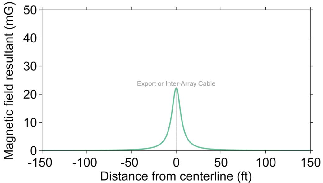
Figure 4. Magnetic field around the Inter-Array or Export Cables at the seabed at varying distances from the cable centerline assuming a burial depth of 6 feet and no armoring or sheathing.
