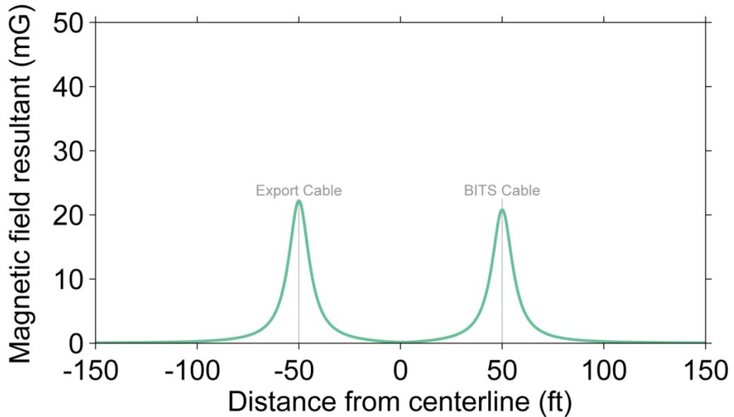
Figure 5. Magnetic field around the parallel Export and BITS Cables at the seabed at varying distances from the cable centerline assuming a burial depth of 6 feet and no armoring or sheathing.
