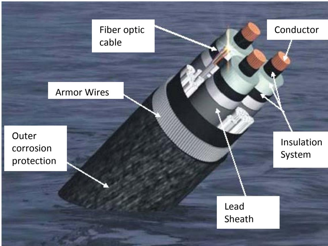
Figure 1. Configuration of an AC Inter-Array, Export, and BITS Cables showing 3-phase conductors and surrounding sheathing.
