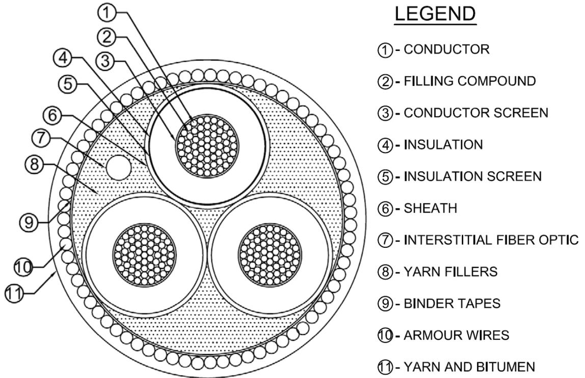
Figure 3. Cross-sectional view of the buried marine Inter-Array, Export, and BITS Cables.
