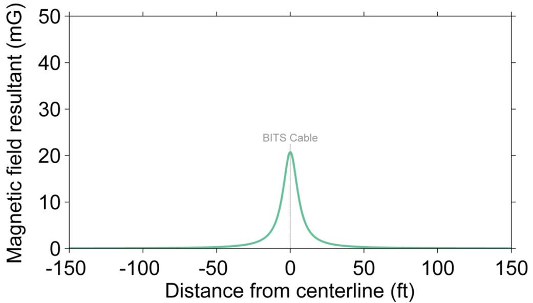
Figure 6. Magnetic field around the BITS Cable at the seabed at varying distances from the cable centerline assuming a burial depth of 6 feet and no armoring or sheathing.
